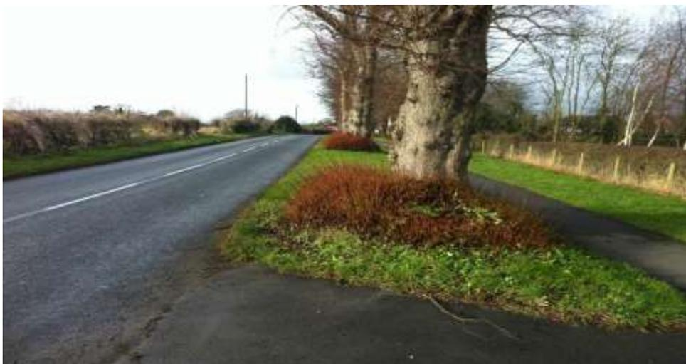
Picture taken from 1.9m above ground level at the same spot and the second tree is within the visibility splay.
